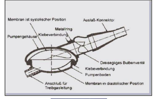
the bloodflow is straightened by using a three leaflet bulb valve for inlet and outlet
